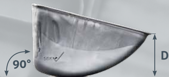
Bucket height front The bucket is placed vertically, and measured from the front and down
