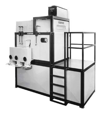
The Combi V is a complete cereal seed cleaning plant consisting of a clipper-de-awner, a cleaning machine and air systems and a short grain indented cylinder.
