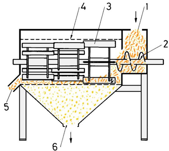
The Hambo is a solid construction, consisting of a frame and a housing of steel, a tripartite rotor with exchangeable beaters, an exchangeable scarifying basket, a driving mechanism with geared motor, and an outlet hopper of steel.
